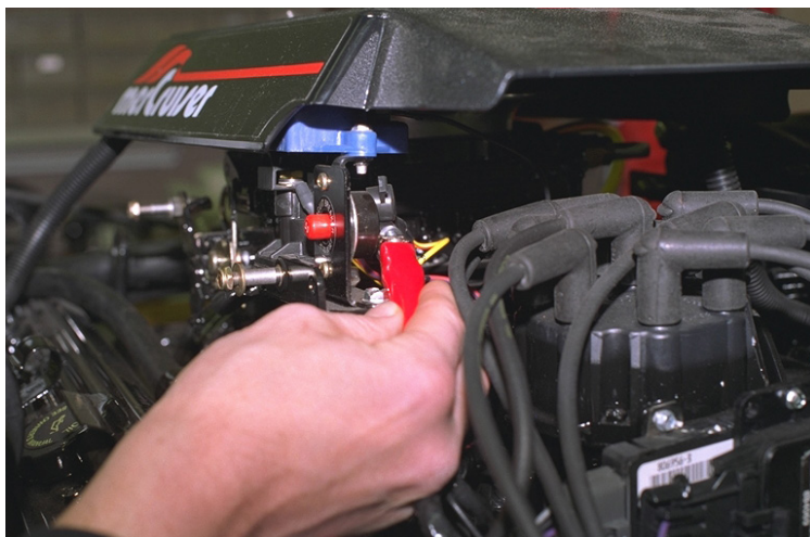
Figure 33 Circuit Breaker Terminal
