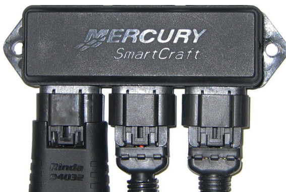
Figure 12 Adapter #94032 attached to junction box
