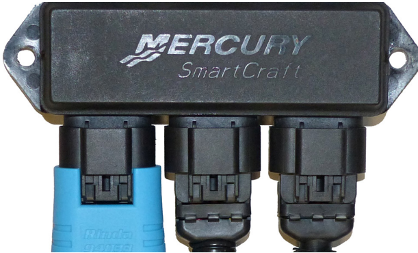
Figure 32 Adapter #94033 attached to junction box
